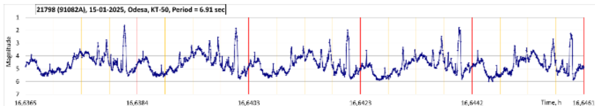
Figure 8. A fragment of the light curve of SC 21798 (91082A, DMSP 5D-2 F11), obtained on 15-01-2025 in Odesa on the KT-50 telescope in tracking mode. The apparent rotation period is 6.91 sec (it is marked with vertical lines on the light curve).
