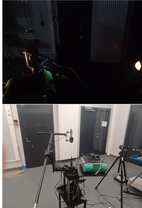
Figure 3. The goniometer in action and after action. The light source is on the right, the green-grey box is the ASD FieldSpec 4 spectroradiometer, the fore optics with the rotating polariser is on the arm, and three rotating motors with their controllers in the centre.
