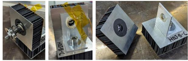
Figure 16. Ejected screw and separated panels of the B-C sample after testing.
