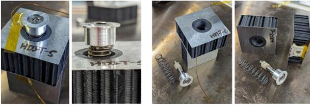
Figure 18. Ejected screw and separated panels of the HDJ-T-S sample (left) and HDJ-T-C (right) sample after testing.
