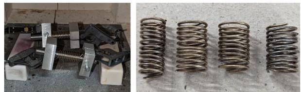
Figure 12. Spring fabrication setup inside the oven before heating (left). SMA springs post-heating (right).
