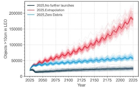
Figure 9. Number of objects > 10 cm in LEO in the simulated scenarios of long-term evolution of the environment over 200 years.
