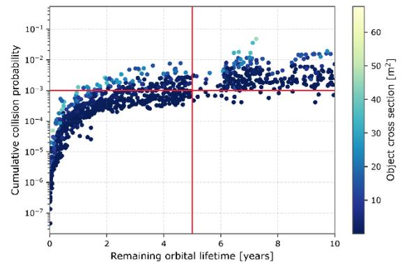
Figure 8. Relationship between orbital lifetime and cumulative collision probability for the objects in the end-of-life pipeline. ESA requirement thresholds depicted in red: 5-year lifetime limit and 1-in-1000 cumulative collision probability.
