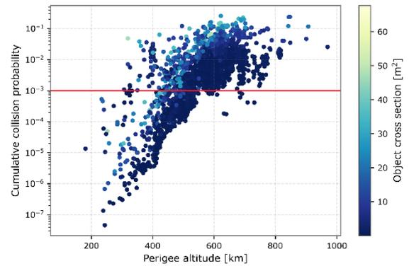
Figure 7. Cumulative collision probability as a function of perigee altitude for the objects in the end-of-life pipeline. ESA requirement threshold depicted in red: 1-in-1000 cumulative collision probability.
