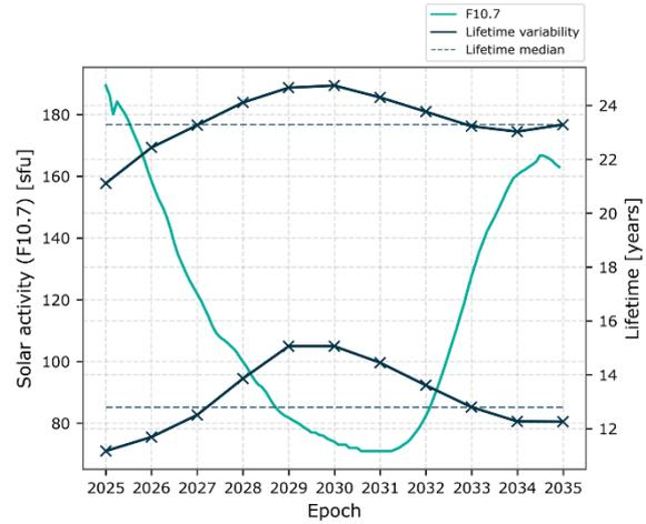
Figure 2. Variation of remaining orbital lifetime with the solar cycle. Solar cycle, represented by the solar radio flux at 10.7 cm, shown in green. Variation in lifetime of two objects, and their associated median lifetime, shown in dark blue.
