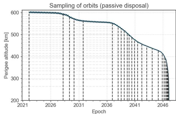
Figure 3. Discretised trajectory for cumulative collision probability computation. Discretisation based on 10 km change in perigee altitude.
