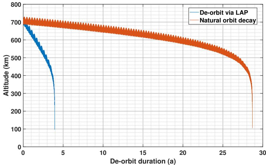
Figure 4. Comparison of the altitude over time curves of the de-orbiting of an 800 kg satellite from a 700 km orbit as a result of the simulations in GMAT. It shows clearly the decreased de-orbit time of 3.8 years for the active de-orbit via LAP in relation to 28 years for the natural orbit decay.
