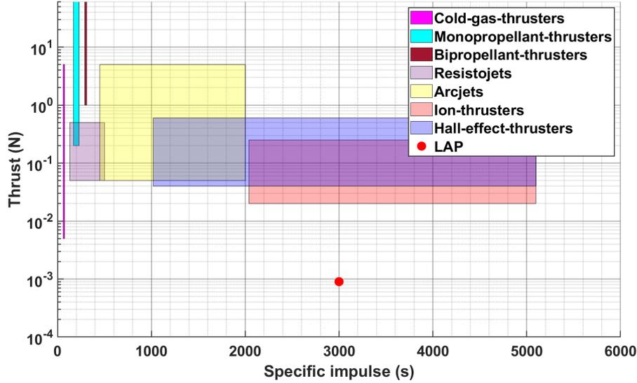
Figure 2. The performance parameters thrust and specific impulse shown in comparison to typical ranges of chemical propulsion systems (cold-gas-thrusters, monopropellant-thrusters, bipropellant-thrusters) according to [9] and electric thrusters (resistojets, arcjets, ion-thrusters, hall-effect-thrusters) according to [10]. From the technologies mentioned above, at the moment only monopropellant-, bipropellant-, ion-, and hall-effect-thrusters are seen as suitable for the purpose of de-orbiting.
