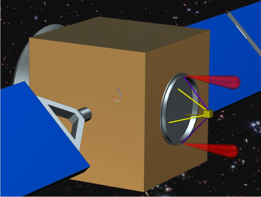
Figure 3. Spacecraft with LAP-unit. Visible is the deployed boom, shown in yellow, consisting of three struts, mounted in the center of the launch adapter with the scanning unit at the end. The plumes formed from ablated material are shown in red. The symbolized laser beams are shown in purple and for the sake of visibility hugely over-sized.
