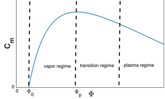
Figure 1. Principle sketch to visualize the influence of the fluence  $\Phi$  on the momentum coupling coefficient  $C_m$ , described in [1], where  $C_m$  increases after the threshold fluence  $\Phi_0$  is surpassed with a maximum of  $C_m$  around the plasma threshold  $\Phi_p$ . The decrease of the momentum coupling coefficient, after fluence is surpassing  $\Phi_p$ , occurs due to plasma shielding.
