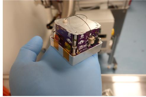
Figure 3. Assembled flight model for SIDLOC-AR6 experiment. (Credit: LSF)
