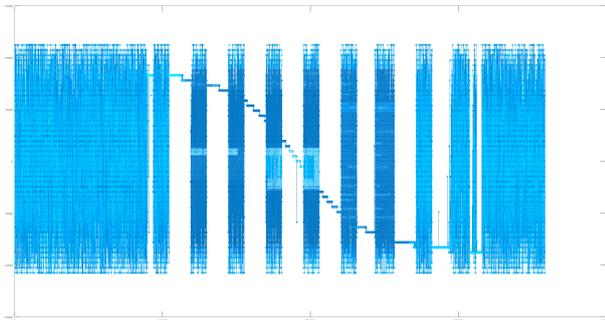
Figure 4. Received DSSS signal showing the Doppler curve. (Credit: LSF)
