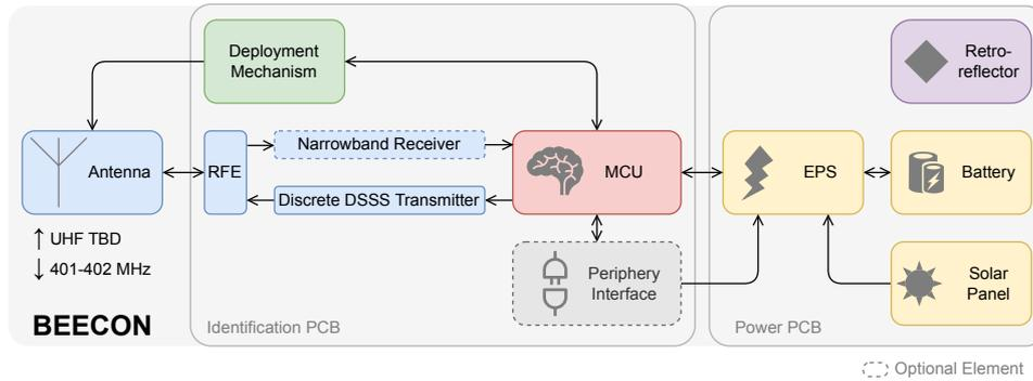
Figure 5. Block diagram of the BEECON design.
