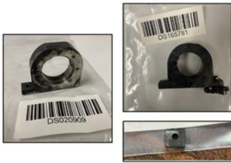
Figure 3. Titanium Fragments (After Impact)
