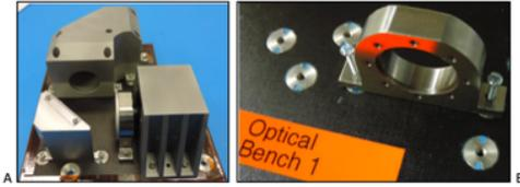
Figure 2. Titanium Camera Mounts (Before Impact)
