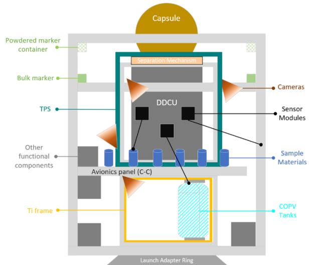
Figure 2. DRACO configuration layout
