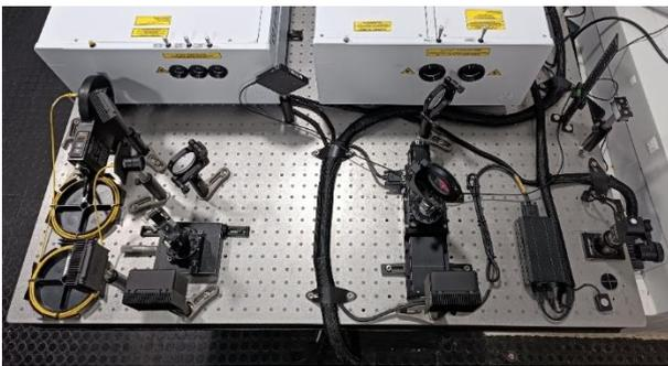
Figure 13. Optomechanics and optical configuration available at the output of the laser benches.
