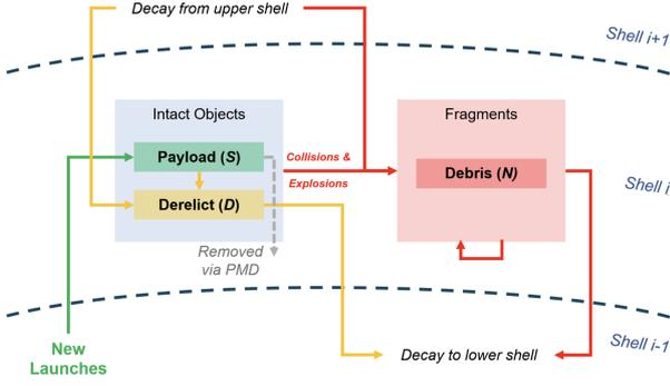
Figure 2. Qualitative schematics of the MOCAT-pySSEM model
