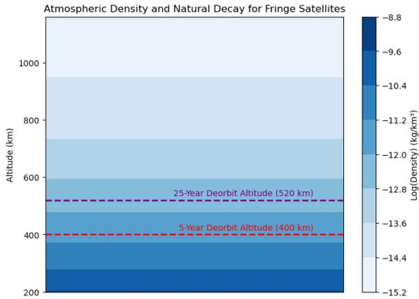
Figure 4. Fringe Satellites Naturally Compliant Orbits, Mass = 220 kg,  $C_d = 2.2$ . Atmospheric density values are static through the simulation.
