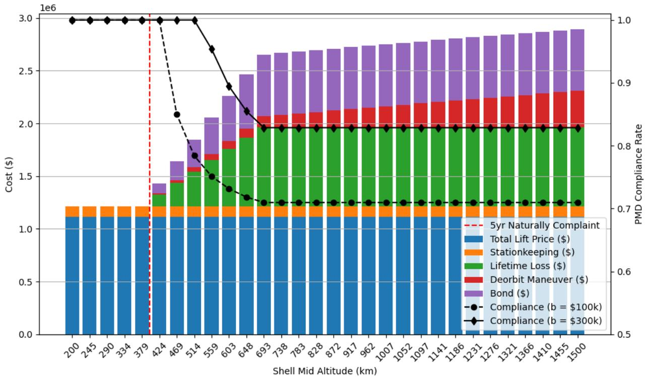
Figure 5. 5yr PMD scenario. For each shell, the total mission cost to the operator is shown. The compliance rate is provided.
