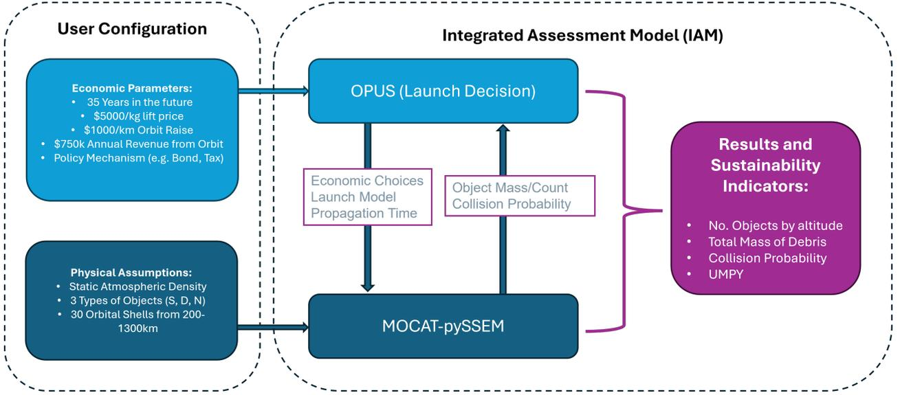
Figure 3. The integration and configuration of OPUS and pySSEM. UMPY is the Undisposed Mass per Year [44].
