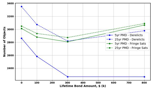
Figure 6. The final number of derelicts and fringe satellites from a 25 year simulation, as the bond increases to \$800k.
