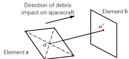
Figure 9 Schematic of judging panel shielding
