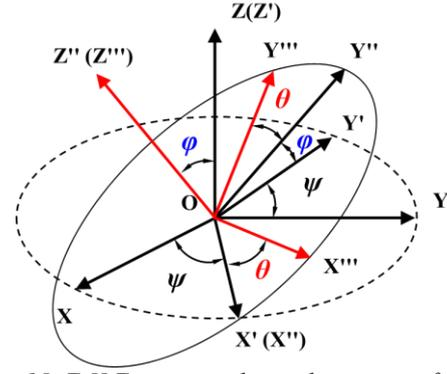
Figure 15 Z-X-Z sequential coordinate transformation
