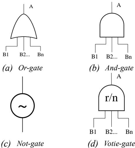
Figure 20 Fault tree logic gate symbols
