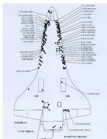
Figure 1 Distribution of impact craters on the surface of space shuttle after mission STS-91
