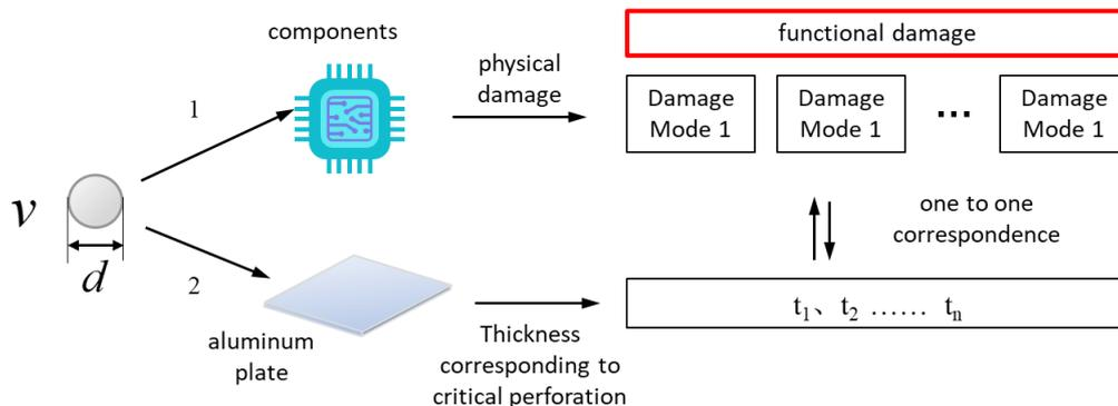
Figure 17 Schematic of damage equivalent model of functional components
