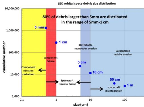
Figure 3 Distribution of quantity with varying sizes of space debris in Low Earth orbit(LEO)<sup>[6]</sup>
