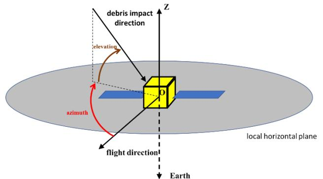
Figure 14 Coordinate system of space debris infow
