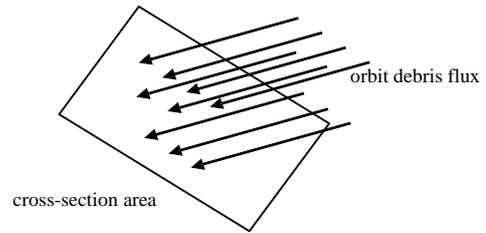
Figure 16 Definition of space debris flux
