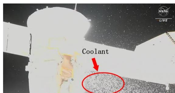
Figure 2 Coolant leakage accident caused by impact of "MS-22"
