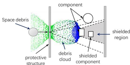
Figure 11 Schematic of shielding analysis based on debris cloud model
