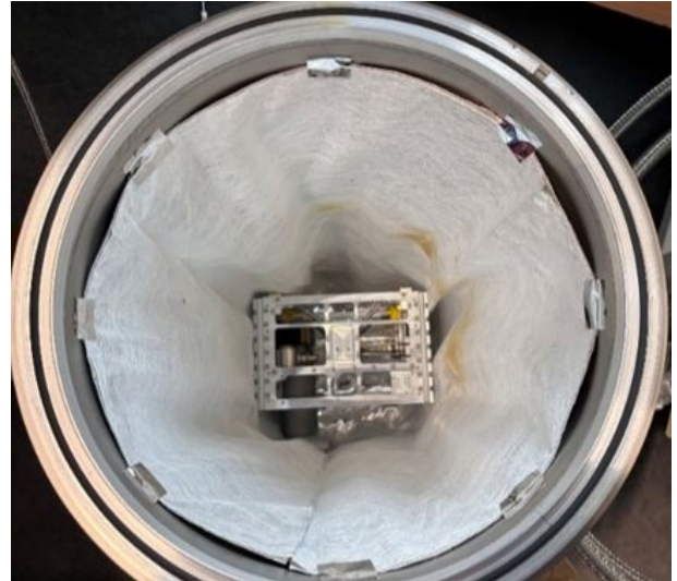
Figure 3. DMM in the vacuum cylinder in the leakage test.
