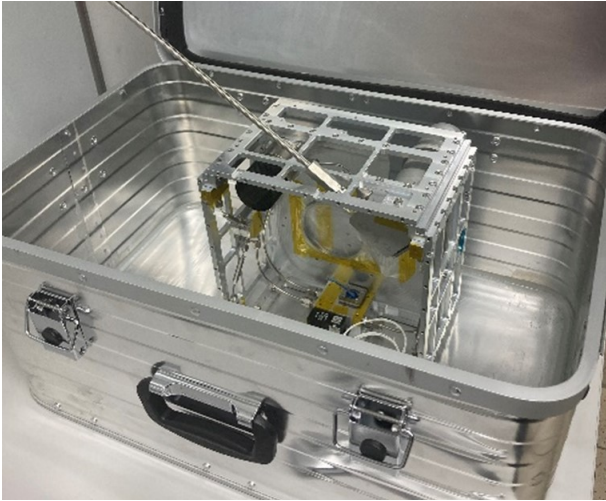
Figure 2. DMM in its containment box during the proof pressure test.
