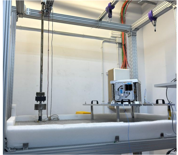
Figure 6. DD in the shock test setup at SENER facilities.
