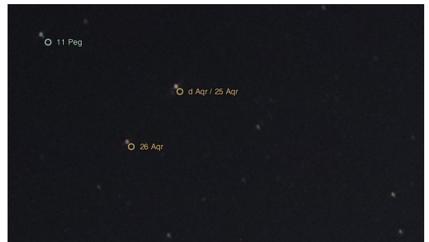
Figure 5. Full field calibration results, zoomed in detail showing that peripheral stars in the top left corner are not properly matched by the calibrated model.
