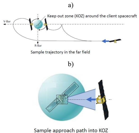
Figure 6. Basic concept of safe rendezvous trajectory
