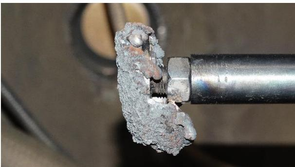
Figure 5. Stainless-steel sample tested in L2K
