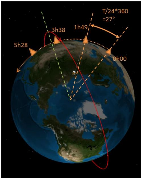
Figure 10: Base positions at different times of debris passage at its ascending node
