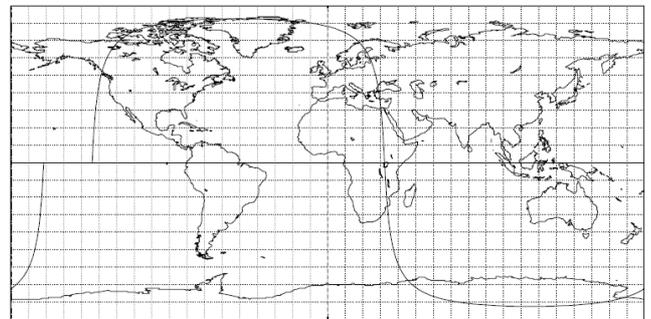
Figure 8: Ground track of satellite METEOP on an orbit (altitude 1195 km, inclination 82.6°, period 1h49', nb rev/day 13.16), shift at the equator: 3059 km
