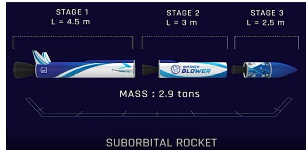
*Figure 4: Dimensions of the different rocket stages*
