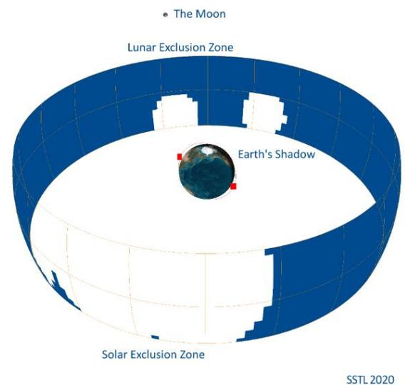
Figure 12: Instantaneous coverage of GEO from two LEO SSA Satellites
