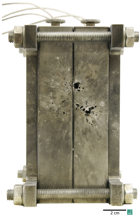
Figure 11. Mechanical damage to battery front side in experiments 4763.
