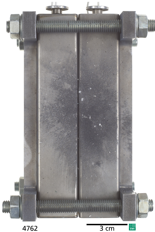
Figure 10. Mechanical damage to battery front side in experiments 4762.
