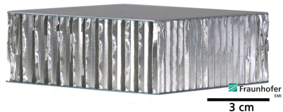
Figure 3. Photograph of aluminum honeycomb sandwich panel used to shield the batteries.
