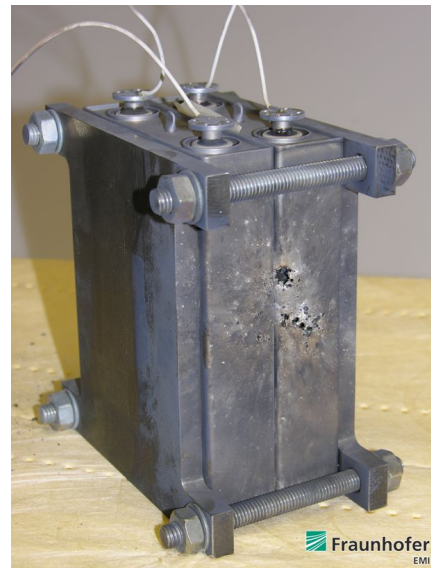
Figure 1. Nickel cadmium battery cell after hypervelocity impact (exp. 4763).
