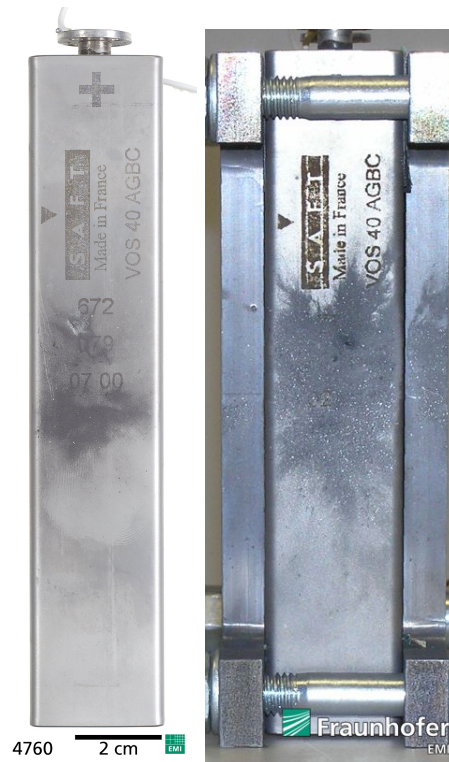
Figure 9. Mechanical damage to battery front side in experiments 4760 (left) and 4761 (right).
