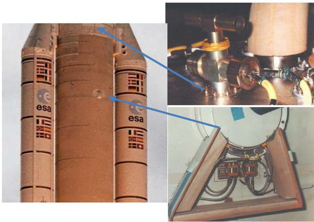
Figure 8. Ariane 5 EPC passivation system
