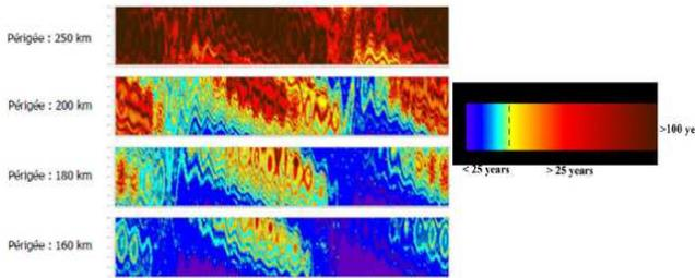
Figure 12. Orbital lifetime of A5 ESCA vs. Perigee
