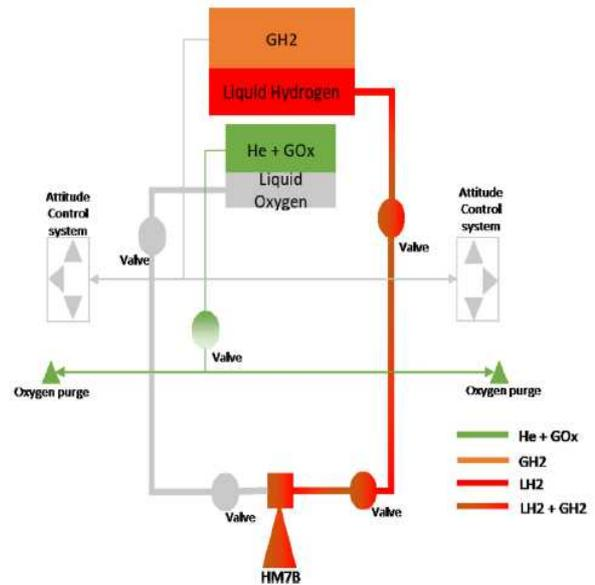
Figure 13. EOLM process for A5 ESCA
