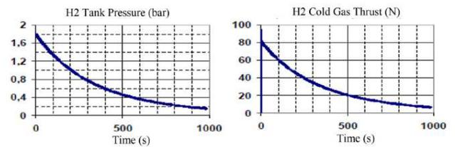
Figure 14. Pressure and thrust evolution on H2 side
