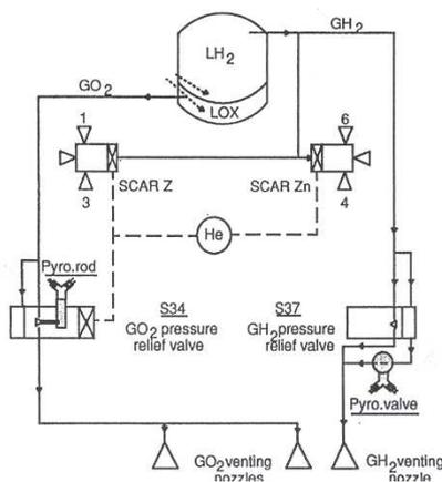
Figure 3. H8-H10 passivation scheme
