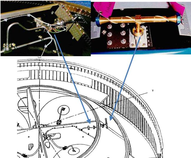
Figure 5. Ariane 5 EPS passivation scheme
