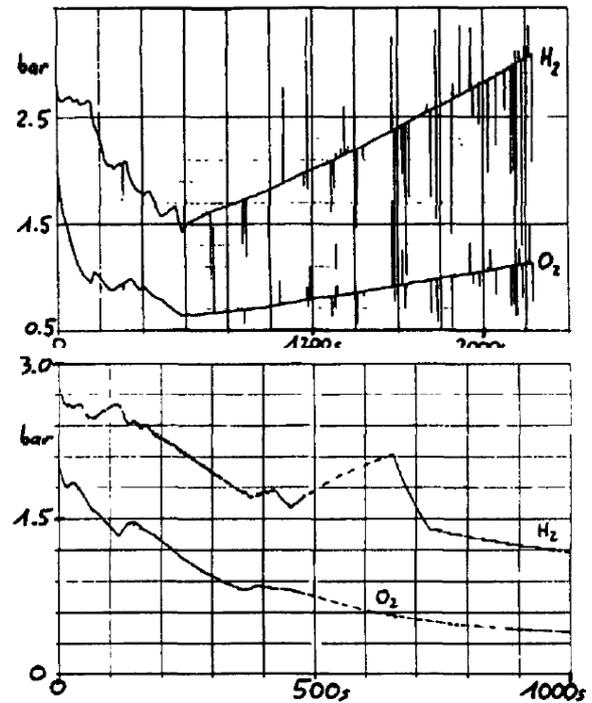
Figure 4. H8-H10 pressure evolution without (top) and with (bottom) passivation
