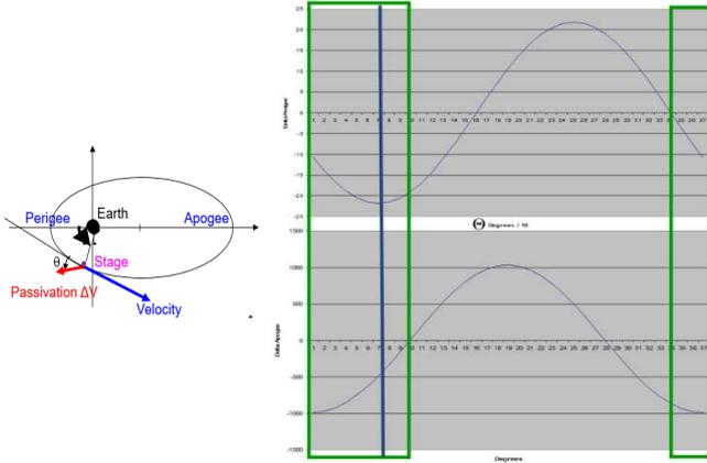
Figure 11. A5 ESCA EOLM principle. Perigee (top) and Apogee (bottom) modification
