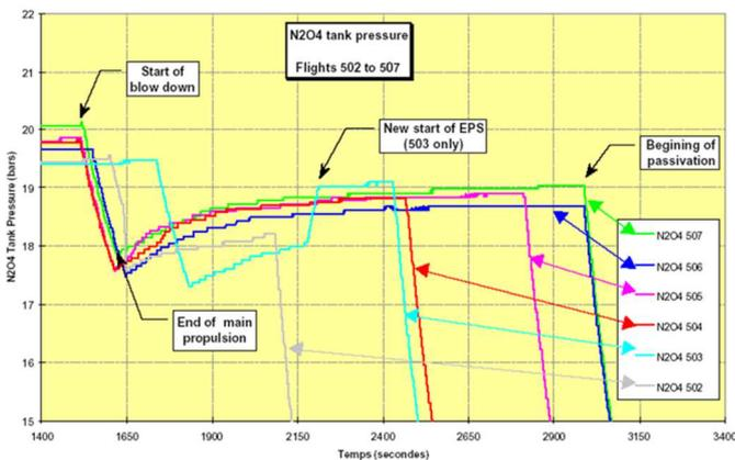
Figure 6. Ariane 5 EPS pressure evolution with passivation (N2O4 side)
