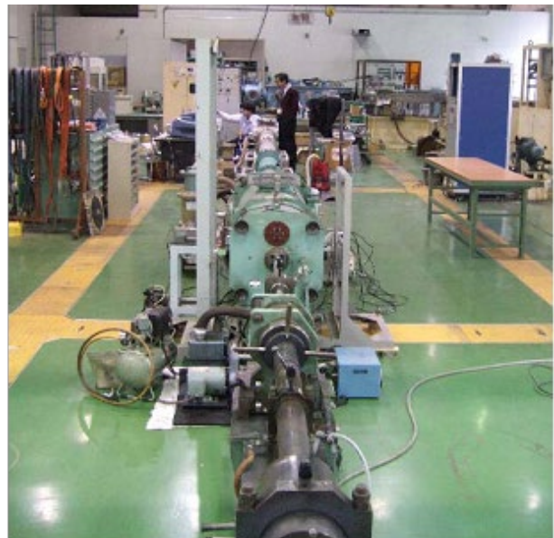
Figure 3. Two-stage light-gas gun at ISAS/JAXA
