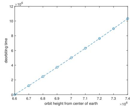
Figure 4. Time of de-orbiting versus altitude object 2
