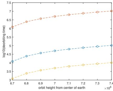
Figure 6. Time of de-orbiting versus altitude for all 3 objects in logarithmic scale
