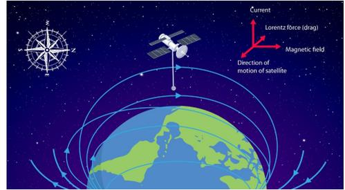
Figure 1. Force on a single long tether.
