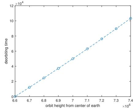
Figure 3. Time of de-orbiting versus altitude object 1
