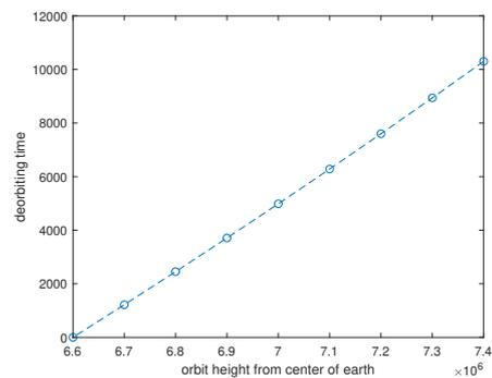
Figure 5. Time of de-orbiting versus altitude for object 3
