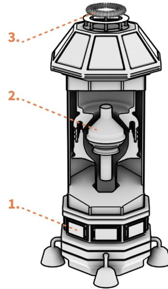
Figure 12. Pulverisation of collected space debris through (3) a rotating cutter head drill and (2) a cone crusher. The pulverised material is stored in (1) service vehicles connected to the chaser spacecraft.
