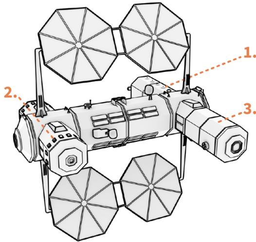
Figure 14. The Space Recycling Facility consists of a module to (2) separate the collected raw material composite, (1) conduct material analysis and (3) manufacture products on demand.
