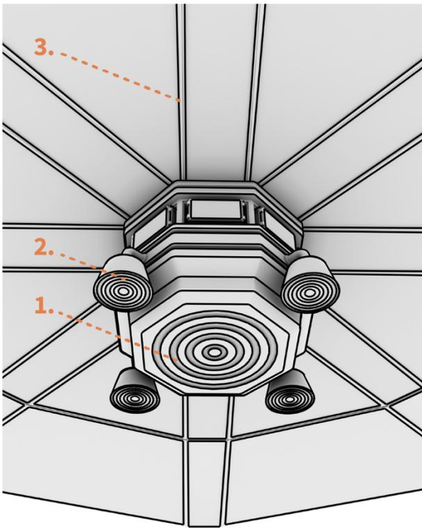
Figure 10. The *Space Vulture* chaser spacecraft is propelled by (1) a high-power solar electric propulsion system (2) that ensures controlled de-orbiting to capture debris. (3) An origami solar array is deployed to produce the electricity needed for solar electric propulsion.
