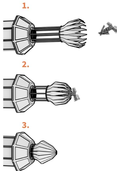
Figure 11. The multi-arm robotics-based system is designed to (1) target, (2) chase, and (3) capture debris.
