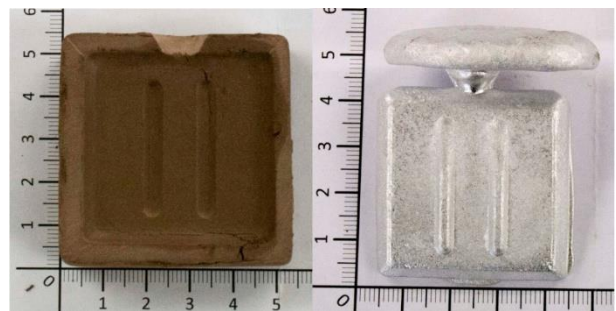
Figure 2: (Left) Sintered regolith simulant mould and (Right) resulting aluminium casting, J. Baasch, TU Braunschweig / TU Berlin
