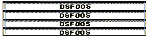
Figure 9. Indexer Slip Example. The blue vertical reference lines reveal a varying drift of several millimeters along the travel direction of four successive images of a 1.22-meter panel. The indexer (above the alphanumeric panel ID) allows the images to be aligned to 70-micron tolerance in the lateral direction. Coupled with the cross-tunnel registration assured by precision mounting techniques, these steps enable image stacking of multiple exposures to achieve enormous signal-to-noise improvement, and to assure that the two perspective views are exactly aligned so that millimeter-scale fragments can be exactly surveyed within the entire panel expanse.
