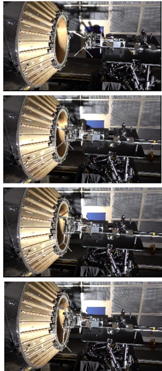
Figure 4. Initial experiment of BBM1 capturing PAF
