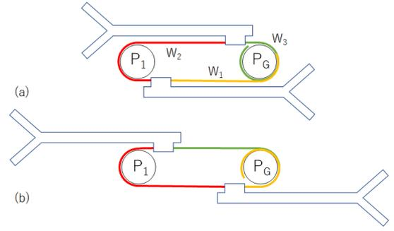
Figure 12. Wire routing design (a) contractile state (b) extending state
