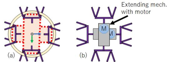
Figure 9. Configuration of (a) IFO satisfying V shaped structure, and (b) its equipment configuration.
