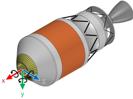
Figure 5. Coordinate definition. Origin is at the center of PAF.
