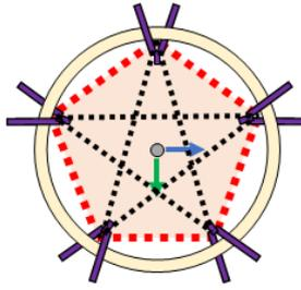
Figure 7. Configuration of the PAF capturing by 5 V shaped structure. Black line describes the connection of gripping point when 1 set has failed.
