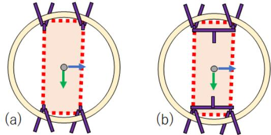
Figure 8. Configuration of the PAF capturing by 4 V shaped structure. (a) 4 extending mechanism (b) 2 extending mechanism.
