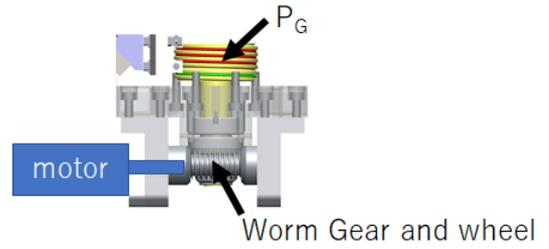
Figure 13. Cross section of the motor, Pulley  $P_G$ , and worm gear.
