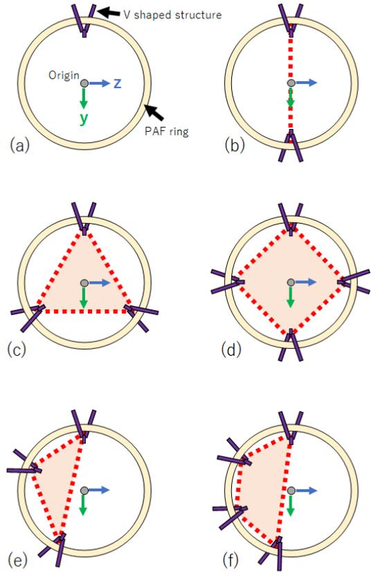
Figure 6. Configuration of the PAF capturing by 1 to 4 V shaped structure.
