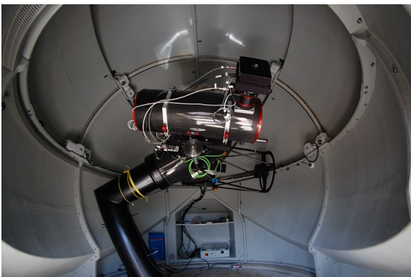
Figure 3. Dome, mount, 25 cm telescope (foreground), and 50 cm telescope (background), SMART-02-KENT, by courtesy of J. Herzog
