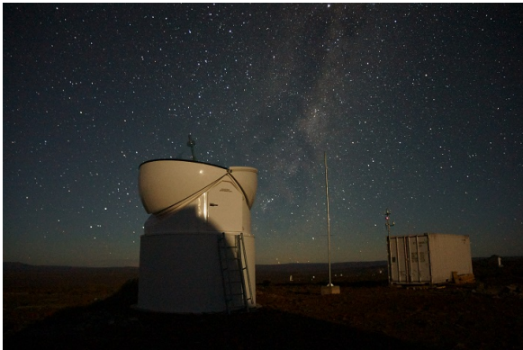
Figure 1. Telescope station SMART-01-SUTH with dome, lightning rod, and container, by courtesy of H. Fiedler
