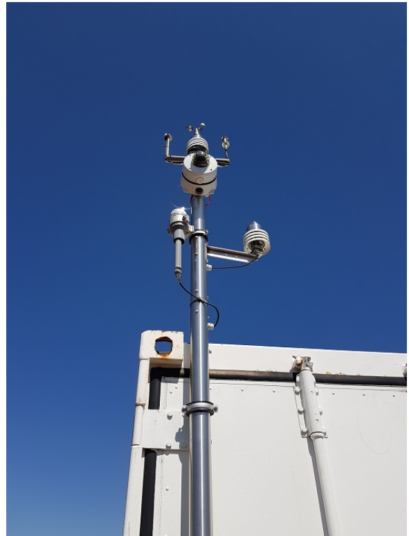
Figure 4. Weather station, GPS antenna, and webcam towards the dome, altogether mounted on a pole at the container, SMART-01-SUTH, by courtesy of J. Bernardo (SAAO)
