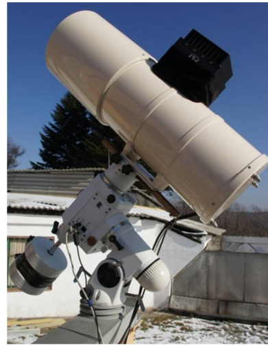
Figure 3. 22-cm survey ORI-22 telescope on automated EQ6-Pro mount in Ussuriysk (Far East, Russia)
