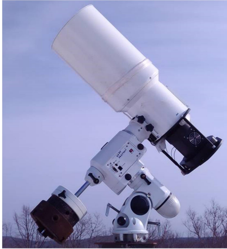
Figure 5. 19.2-cm VT-78a telescope on automated EQ6-Pro mount in Ussuriysk (Far East, Russia)
