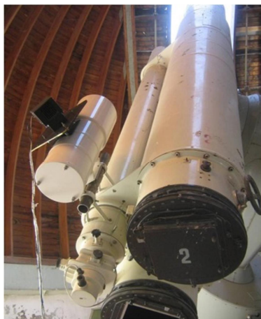
Figure 2. 22-cm survey ORI-22 telescope installed on 40-cm double Zeiss astrograph in Kitab (Uzbekistan)
