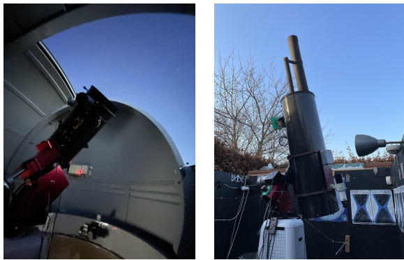
Figure 5. Rantiga Observatory to the left and Solaris Observatory to the right. Diaphragm with straylight reducing tubes visible in the right image.
