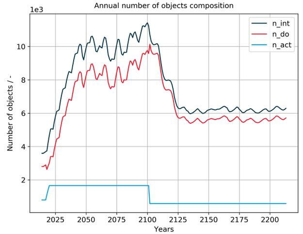
Figure 1. Evolution of the number of intact objects over the time span of 200 years of a simulation scenario with a large constellation. The number of active spacecraft was iteratively re-calculated from the scenario definition.
