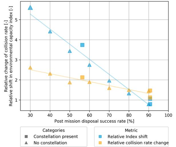
Figure 7. Comparison of relative shift of the index (light blue) and relative change in collision rate (yellow) between the beginning and the end of the debris simulation.
