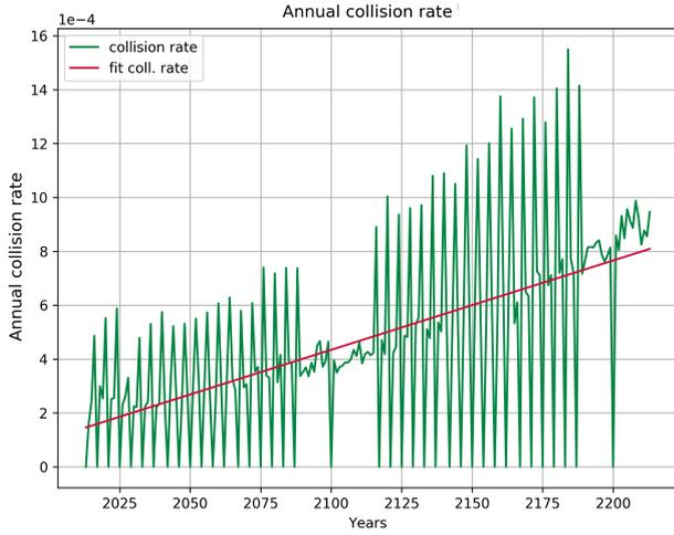
Figure 2. Annual collision rate evolution of a DELTA simulation with a high launch rate of small payload. (ISTS campaign, scenario 27).
