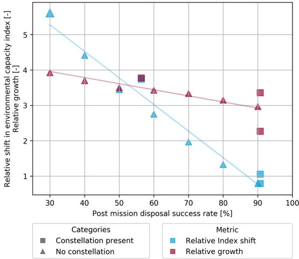
Figure 6. Comparison of relative shift of the index (light blue) and relative growth in number of objects (purple) calculated with respect to the beginning and the end of the debris simulation. The larger separation of the data points for the index allows for a better discrimination of the different prevalent PMD rates in the simulations.
