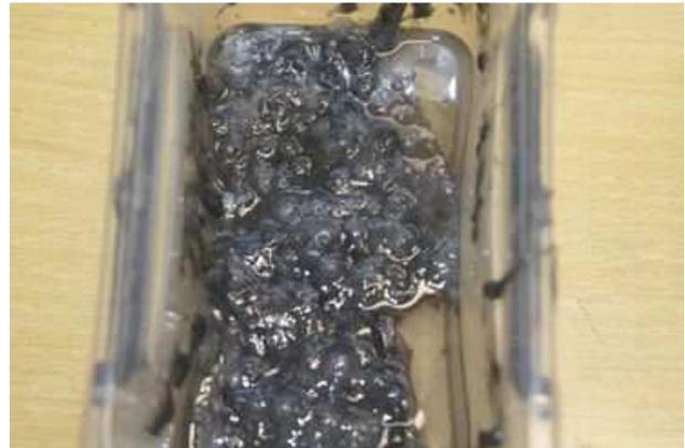
Figure 4-1. Polystyrene part floating on an acetone bath.
