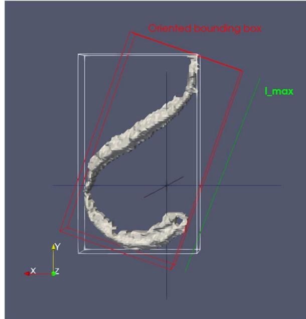
Figure 4-13. Bounding box calculation in view of characteristic length calculation.
