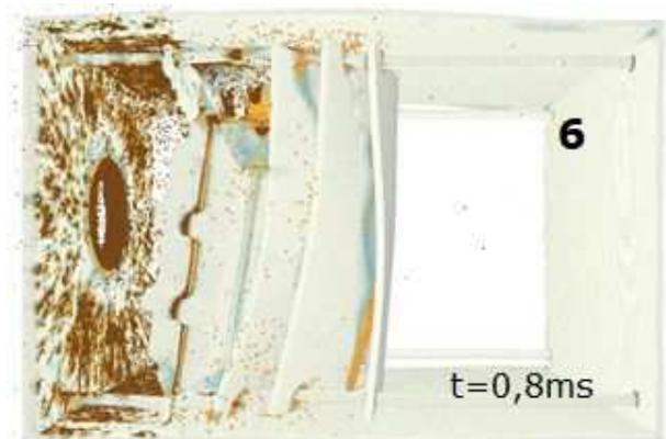
Figure 5-3. Top view of plastic strain inside the structure (see also fig. 3-7 for inner impacts on the front face)
