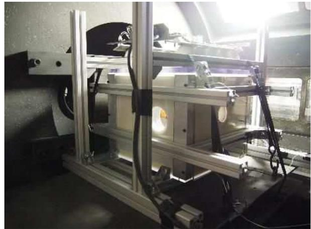
Figure 3-3. Container in the impact chamber (projectile launched from the right side)
