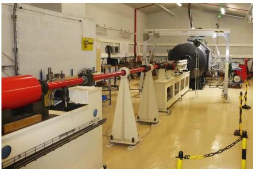
Figure 3-2. HERMES launcher and its impact chamber, in black
