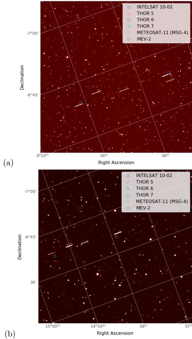
Figure 5: On the left, observation of Intelsat 10-12 and MEV-2 during the close approach (on 2021/04/05) and on the right, one object is visible after the docking (on 2021/04/12). Circles provide the positions computed from last TLE.
