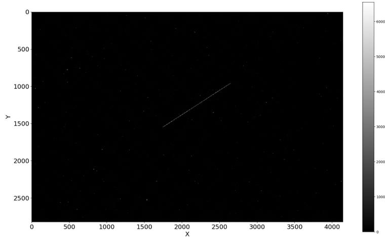
Figure 4: Light streak obtained for SL-14 (norad 20511) at 630 km of altitude observed from our Normandy observatory with a RASA-8 telescope. Exposure time is 1 s. The  $x$  and  $y$  axis represent the camera pixels.
