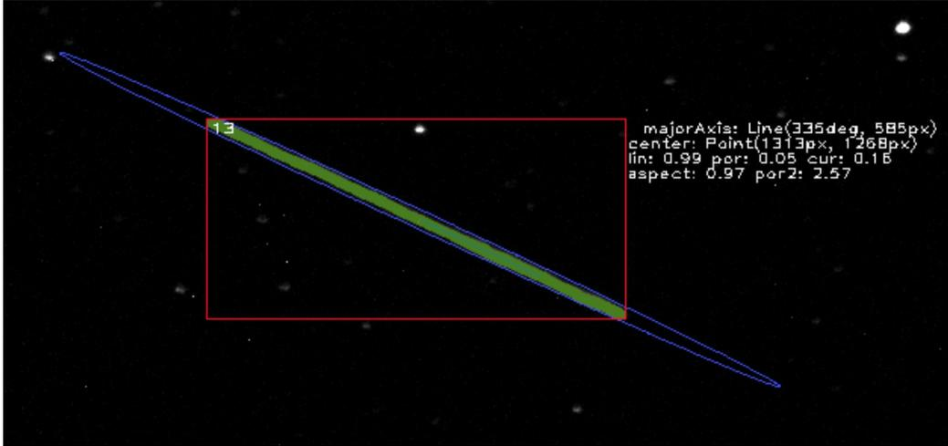
Figure 2: Streak detected with the software. The streak features are displayed directly on the image.
