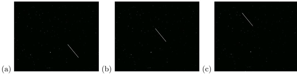
Figure 3: Series of streaks detected for a LEO satellite for a single passage.
