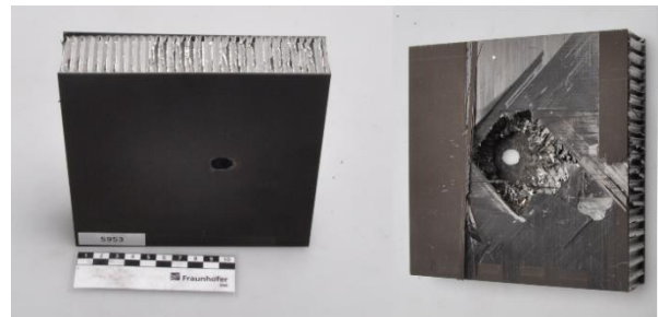
Figure 2. CFRP honeycomb sandwich panel after an impact with a 5.5 mm aluminium sphere at 7.0 km/s.
