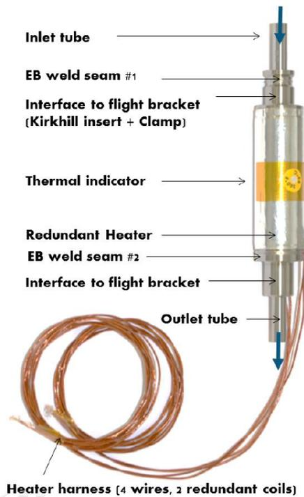
Figure 4: Airbus Safran Launchers SMA valve
