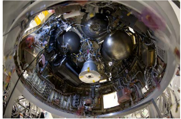
Figure 23. Open view of the AVUM components and tanks.
