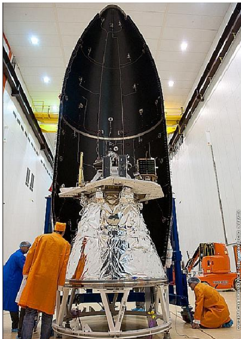
Figure 2. AVUM with LARES-A&H/SS platform. ALMASat and the Cubesats dispensers are also visible.
