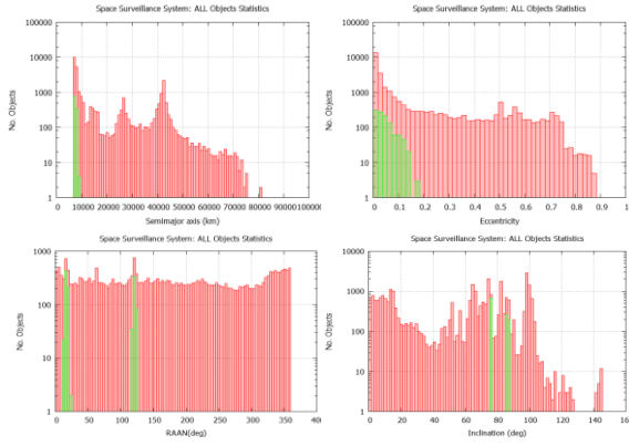
Figure 2: Histograms of all objects from MASTER baseline + fragments from collision LEO inserted in the baseline population, from top to bottom and from left to right: number of objects versus semimajor axis, eccentricity, RAAN and inclination
