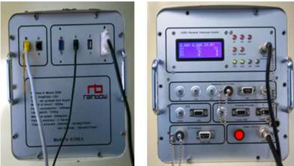
Figure 6. Telescope control units of the OWL-Net imbedded in the mount
