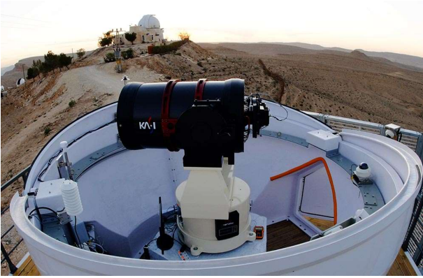
Figure 5. Telescope system (optical tube assembly and mount) of the OWL-Net installed in Israel site
