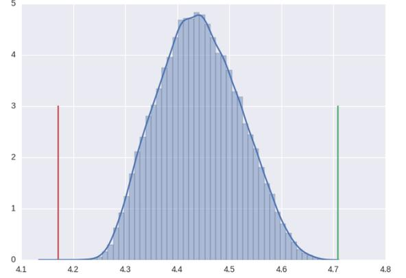
Figure 5. Distribution of the latitude with the reliable impact zone estimation with the impact interval boundary
