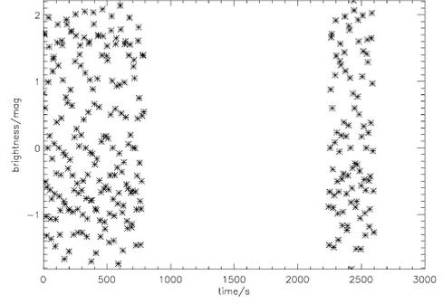
Figure 2. Relative magnitude of rocket body 16528 with linear trend eliminated.
