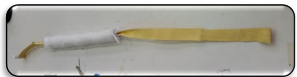
Figure 23- 5 silica layers as thermal insulation material before the insertion inside the 3M Nextel sleeve
