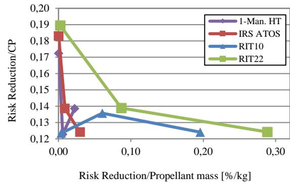
Figure 15: Comparison of the risk reduction by collision probability against risk reduction by propellant mass
