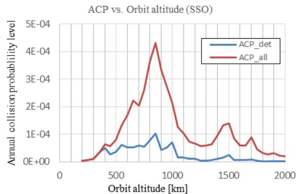
Figure 7: Annual Collision Probability Level for different orbit altitudes for SSO (Source: DRAMA-2.0)
