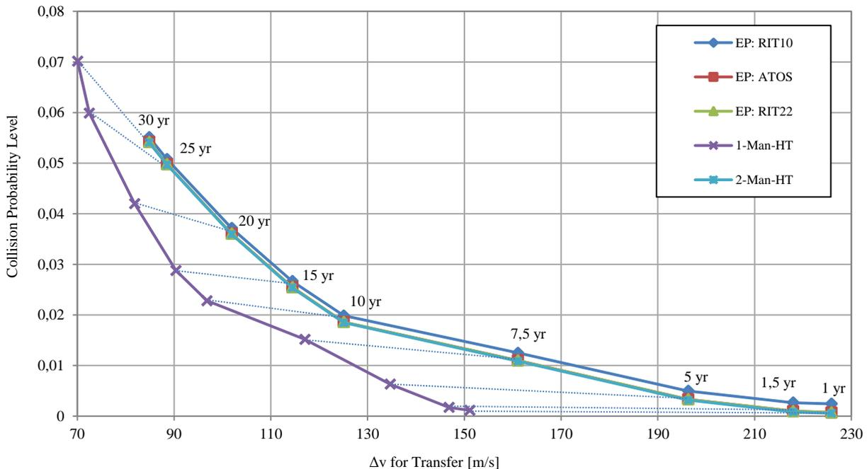
Figure 13: Collision probability and  $\Delta v$ -requirements for different PMD durations and manoeuvre types (Source: DRAMA-2.0)
