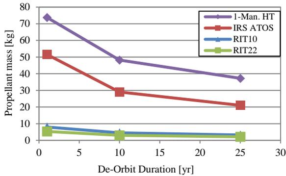
Figure 14: Propellant mass for different propulsion types
