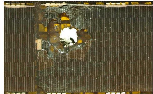
Figure 7 The boundary effect of solar cell after impact
