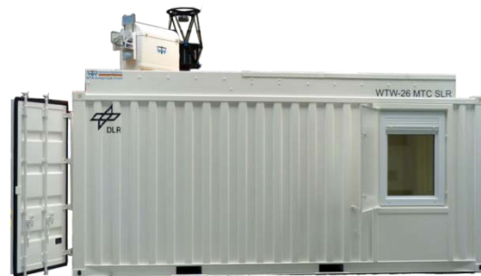
Figure 3. The entire hardware of the transportable laser ranging station is built into a standard 20ft ISO-container. On one end of the container is a platform that raises a bi-static setup on an alt-azimuth mount above the roof of the container. A 17inch telescope is used of the tracking and ranging (further details, see text).
