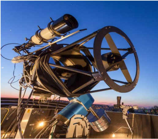
Figure 2. At UFO a bi-static setup is assembled on an equatorial mount. On top of the main 17inch telescope is an auxiliary telescope with an aperture of 10cm. For the ranging the pulses are guided by a passive optical fiber to the auxiliary telescope.
