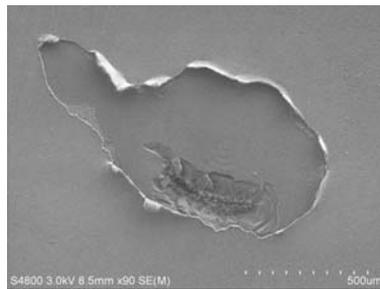
Fig.2 Morphology of the flyer target – a hole caused by a small flyer spalled from the glass basement
