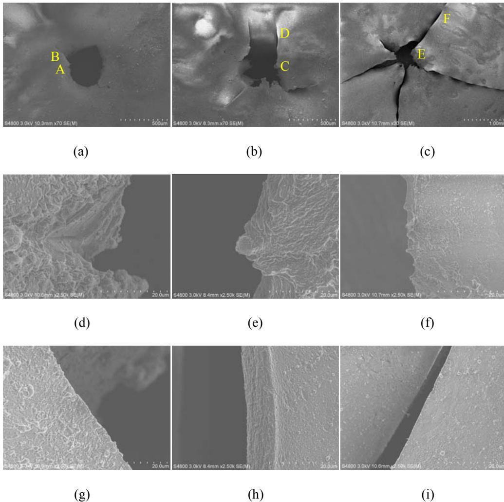
Fig.3 Impact morphology and fracture modes of different polyimide films (flyer velocity of 5.9km/s): (a)25 $\mu$ m film with the tension stress of 0.27MPa; (b) 12.5 $\mu$ m film with the tension stress of 0.27MPa; (c) 8 $\mu$ m film with the tension stress of 0.22MPa; (d)region A; (e)region B; (f)region C; (g)region D; (h)region E; (i)region F
