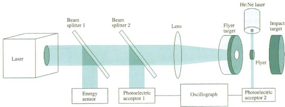
Fig.1 Schematic diagram of the laser driven flyer experiments<sup>[13]</sup>
