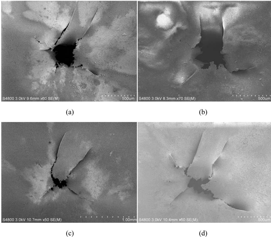
Fig.4 SEM images of the 12.5µm polyimide films at different tension stress (flyer velocity of 5.9km/s): (a)0.06MPa; (b)0.27MPa; (c)1.32MPa; (d)5.24MPa
