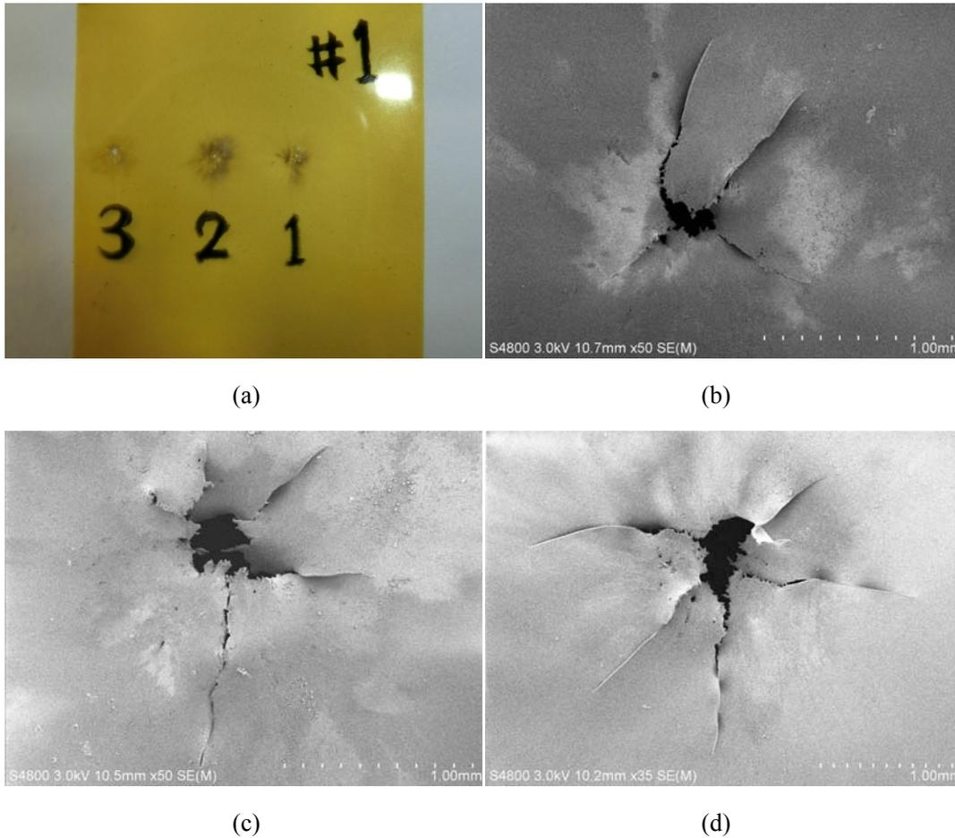
Fig.5 The surface morphology of a 12.5 $\mu\text{m}$ -thick polyimide film impacted successively by 3 flyers at the velocity of 5.9km/s: (a)three impacts on the sample; (b)the first impact; (c) the second impact; (d) the third impact
