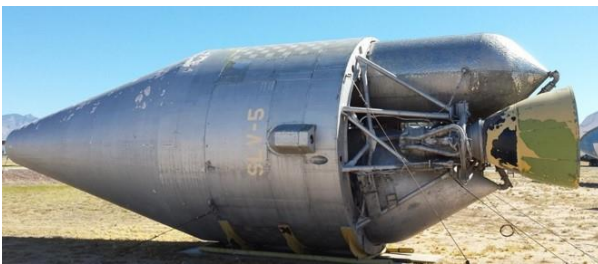
Figure 3: Titan Transtage rocket body test article, recently moved to NASA Johnson Space Center for studies by NASA’s Orbital Debris Program Office. Note that the majority of the original surface is painted white with much of the yellow primer paint of the rocket’s nozzle now weathered away, exposing the original green and blue glass frit surfaces beneath.
