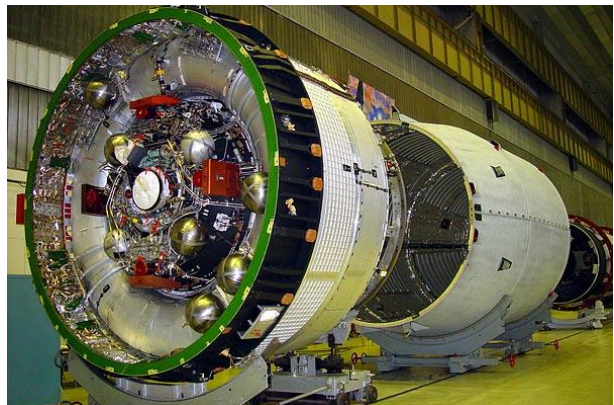
Figure 11: The Briz-M Rocket body [9], believed to be painted mostly white with a black portion near the end of the rocket body, and a section of exposed aluminium. The material types illuminated during the observations are expected to affect the overall shape of the spectrum, which is dependent upon the stage of the rocket body that is observed (e.g. the central portion fully painted white vs. the lower stage with a potential aluminium or carbon or black-MLI or paint signature).
