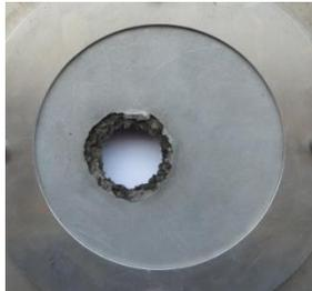
Figure 8. Perforation in the Al/PTFE bumper: Test No.2,  $V_p=5.09$  km/s
