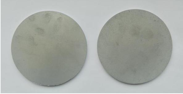
Figure 2. Examples of Al/PTFE sheet: diameter=110mm
