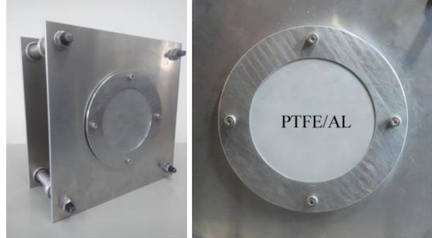
Figure 3. Whipple shield configuration: layout and composition, standoff=10cm
