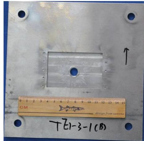
(b) Back Damage of Heat Pipe Back Wall
