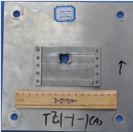
(a) Frontal Damage of Heat Pipe Back Wall
