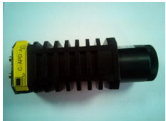
Figure 4 The equipment of APD detector
