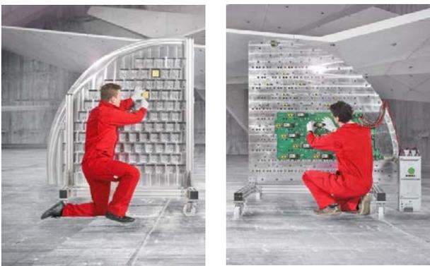
Figure 3 Demonstrator of an antenna quarter, a) front side b) backside with large backplane PCB
