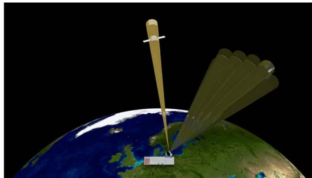
*Figure 1* Beam strategy for track-while-scan mode
