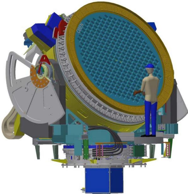
Figure 2 Mechanical model of the antenna with 3-axis-positioner
