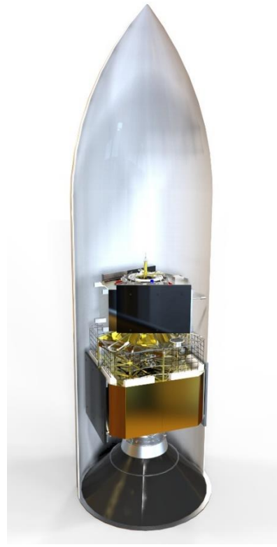
Figure 3: The Necropolis System in Launch Configuration Packaged Within an Ariane Fairing with Hunter Being Stacked on Top of Terminus.
