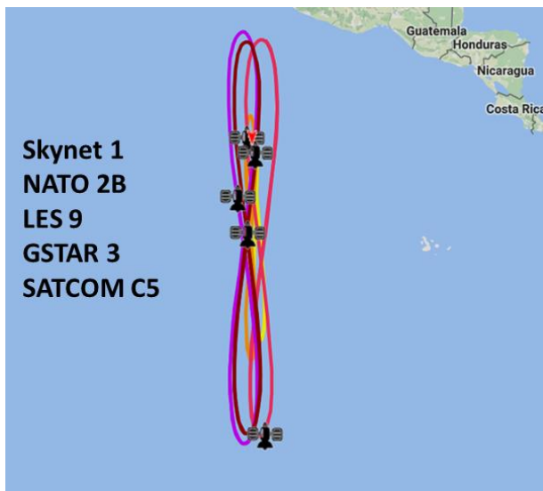
Figure 1: Ground Tracks of 5 of the 53 Satellites at Western Libration Point.
