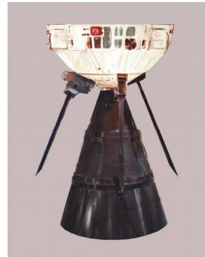
Figure 7. An IUS second stage rocket body as it would likely appear on-orbit. Credit: The Boeing Company (composite by D. Shoots, HX5—Jacobs JETS contract) We can also compare how the model fits a single order fits from one night compared to an averaged spectra of the same order. The two objects, SSN16274 and SSN 27400, were both successfully fit with a one night and multiple night stitches. The multiple night stitches in both cases produced a fit with a worse percentage error but only by an increase of 1%. For SSN16274, this increase is from 0.01% to 1%. For SSN27400, this increase is from 9% to 10%.
